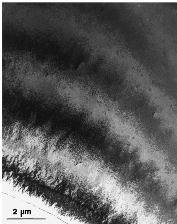
Figure 6 Bright field image with imaging vector \vec{g} = (220) showing a typical example for the mottled contrast behaviour. On the side of the extinction contour closer to the specimen hole, bright spots appear on a dark background, whereas on the thicker side dark spots are superposed to a bright background.
