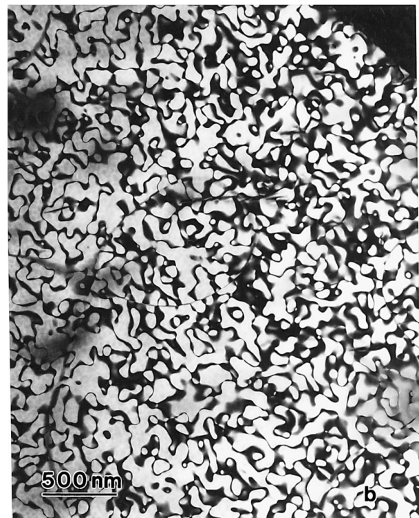
Figure 5 Dark field images of an annealed P9/25 sample obtained in a [011] zone axis (a) with a (200) reflection existing both in the B2 and DO 3 phase, and (b) with a (3 1 1) reflection characteristic for the DO 3 phase. In the second image, only antiphase boundaries (APBs) of the DO 3 -type are visible, whereas in the first case, APBs of the B2-type with much larger domain size dominate.
